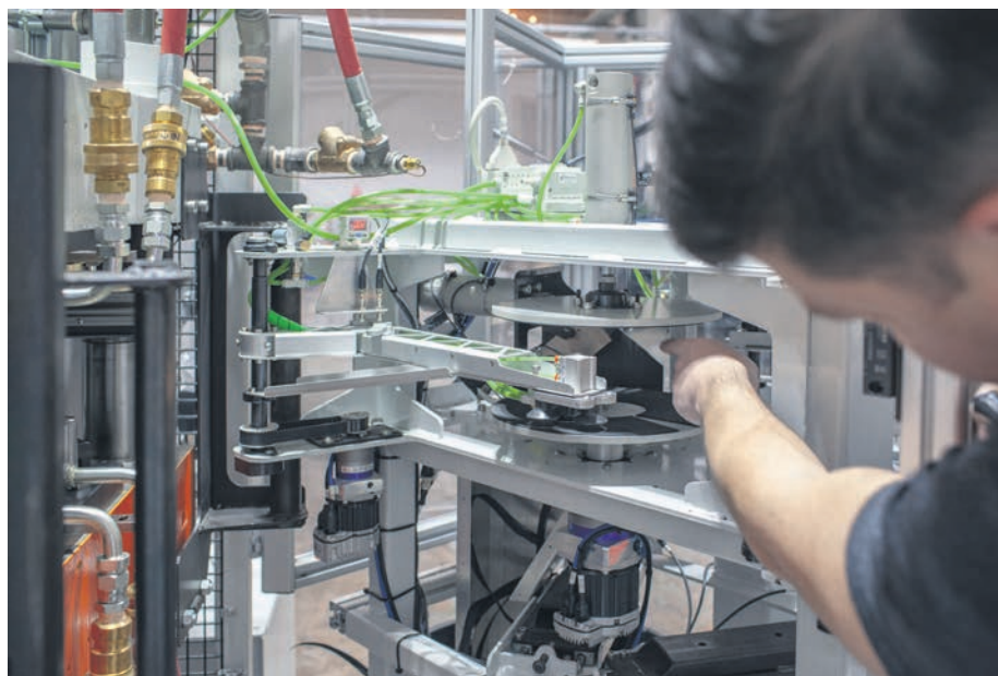
A freshly pressed record rests on the WarmTone's bottom stamper, about to be lifted by a suction arm that grips its center label.
