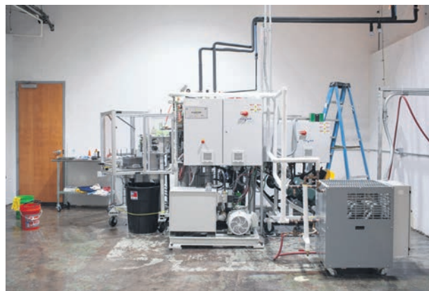
The steamless WarmTone press from Vinyl Technologies takes up surprisingly little space at Smashed Plastic.
